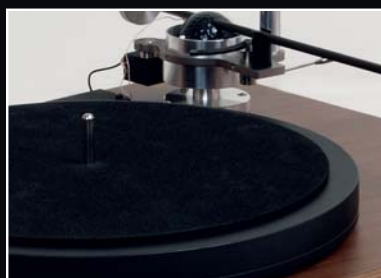
The oversized Delrin platter is nicely finished and gives a nice inert support for your prized vinyl discs...
