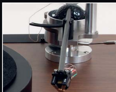
With no way to vary the cartridge overhang, tracking geometry is one thing you don't need to worry about
